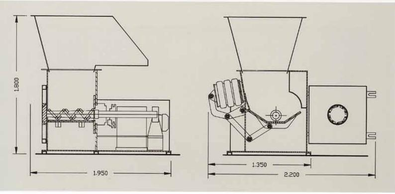
Installed to reduce wires and straps from pulp and wastepaper bales into a convenient and compact roll. Easy to store and commercially viable, it represents a solution to the problem of loose wire around the pulper house. The unit weighs 1380 kgs, is simple to install. Voltage is to your requirements and an air connection of only 1,5 bar is required.
